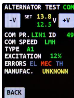
Fig. 7. Diagnostic window of the "COM"-type alternator.
