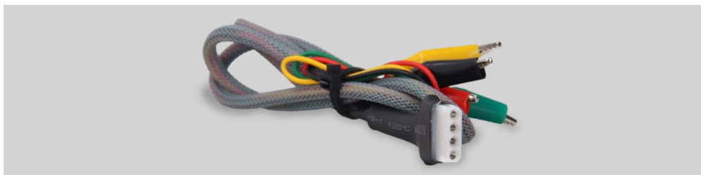
Fig. 4. Four-wire diagnostic cable.
