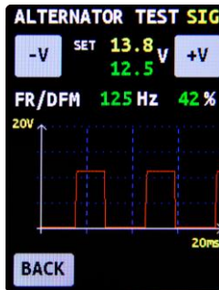
Fig. 8. Alternator diagnostic window when one of the following alternator types "SIG", "RLO", RVC", "C KOR.", "P/D", "C JAP." is selected.
